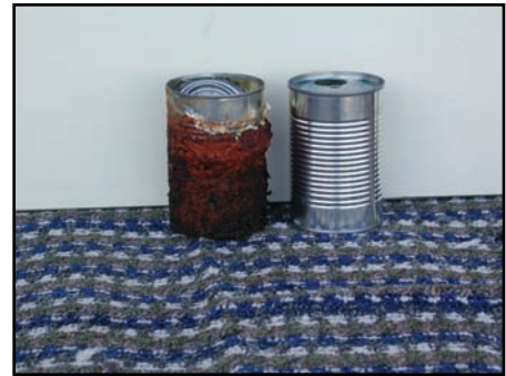
These tin cans were identical until one was used as an anode.
