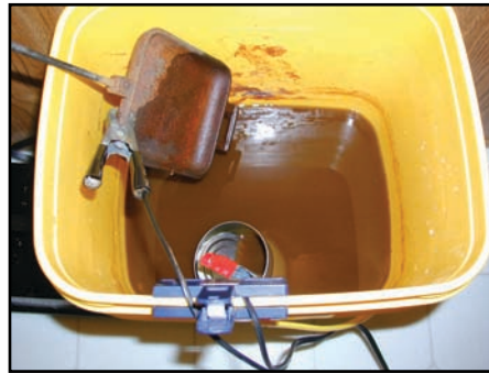
Ready to go! Notice the red clamp is suspended with the clip so it always remains above the waterline.
